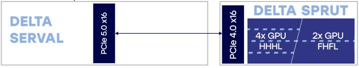
AI, machine learning, HPC and Modeling 1x Server 5x Delta Sprut (1x switching, up to 4x computing), cascade connection
